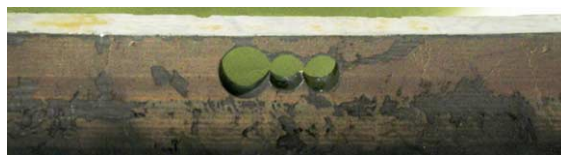
Fig. 2. Plasma exposed side of tile 1BN4 retrieved from JET after the DTE1 campaign. A strong co-deposited zone is visible on the bottom of the tile where it is shadowed from the plasma by tile 3.
